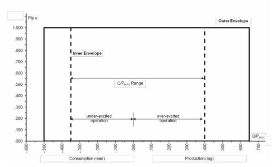
The diagram represents boundaries of a P-Q/Pmax-profile at the connection point by the active power, expressed by the ratio of its actual value and the maximum capacity pu, against the ratio of the reactive power (Q) and the maximum capacity (Pmax). The position, size and shape of the inner envelope are indicative.
