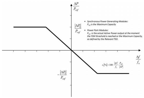
$P_{\text{ref}}$  is the reference active power to which  $\Delta P$  is related.  $\Delta P$  is the change in active power output from the power-generating module. fn is the nominal frequency (50 Hz) in the network and  $\Delta f$  is the frequency deviation in the network.
