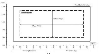
The diagram represents boundaries of a U-Q/Pmax-profile by the voltage at the connection point, expressed by the ratio of its actual value and the reference 1 pu value, against the ratio of the reactive power (Q) and the maximum capacity (Pmax). The position, size and shape of the inner envelope are indicative.
