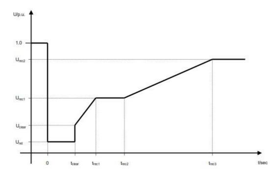
The diagram represents the lower limit of a voltage-against-time profile of the voltage at the connection point, expressed as the ratio of its actual value and its reference 1 pu value before, during and after a fault.  $U_{ret}$  is the retained voltage at the connection point during a fault,  $t_{clear}$  is the instant when the fault has been cleared.  $U_{rec1}$ ,  $U_{rec2}$ ,  $t_{rec2}$  and  $t_{rec3}$  specify certain points of lower limits of voltage recovery after fault clearance.
