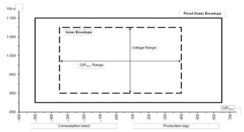
The diagram represents boundaries of a U-Q/Pmax-profile by the voltage at the connection point, expressed by the ratio of its actual value and its reference 1 pu value, against the ratio of the reactive power (Q) and the maximum capacity (Pmax). The position, size and shape of the inner envelope are indicative.
