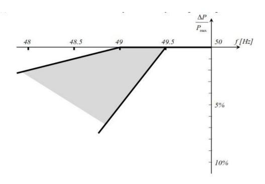
The diagram represents the boundaries in which the capability may be specified by the relevant TSO.
