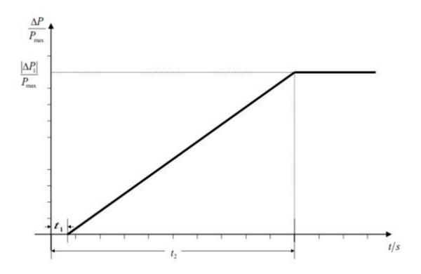
$P_{max}$  is the maximum capacity to which  $\Delta P$  relates.  $\Delta P$  is the change in active power output from the power-generating module. The power-generating module has to provide active power output  $\Delta P$  up to the point  $\Delta P_1$  in accordance with the times  $t_1$  and  $t_2$  with the values of  $\Delta P_1$ ,  $t_1$  and  $t_2$  being specified by the relevant TSO according to Table 5.  $t_1$  is the initial delay.  $t_2$  is the time for full activation.
